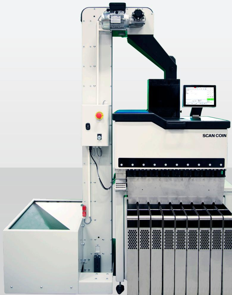
Small and Flexible System with Minimal Footprint that Captures, Stores and Transports Coins
